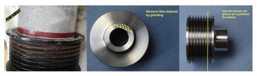
4. **Grinding and cutting the old pulley**. Now, using an angle grinder or other suitable tool, grind flat the front of the pulley until you just – only just – cut through the pulley to reveal the supercharger shaft beneath. You will see when you've nearly ground down to the shaft as the remaining pulley material will become thin and will start to discolour due to heat. Do this all the way back to the where the pulley diameter increases.
