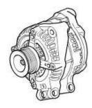
The Generator has a multifunction voltage regulator for use in a 14V charging system with 6÷12 zener diode bridge rectifiers.
