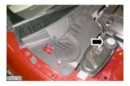
25. Remove the engine cover. Engine Cover (76.11.35)
