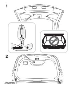
Your vehicle is equipped with a mechanical interior luggage compartment release handle that provides a means of escape for children and adults in the event they become locked inside the luggage compartment.
