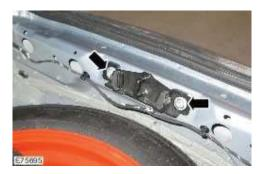
6. Loosen the liftgate to hinge Torx bolts.
