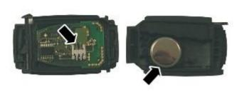
3. Do NOT touch the green printed circuit board, battery or the battery contacts (arrowed in E91988). Oil or contamination on either can affect the key fob performance.
