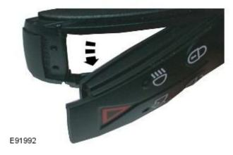
**13.** Remove the silicone pad from the key housing by pushing the silicone pad from the inside of the key housing.
