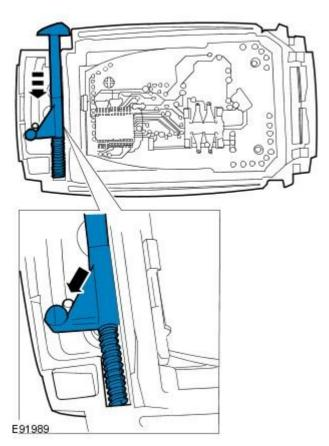
**4.** To replace key blade retaining clip, remove clip (shown in E91989) and install a new clip and spring, ensuring clipping feature is positioned in the front of end stop.
