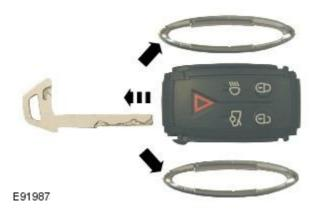
**2.** Remove the two side chrome rings one at a time, by inserting a small, flat-blade screwdriver between the cover and the body, and lightly twisting the screwdriver (see E91987).
