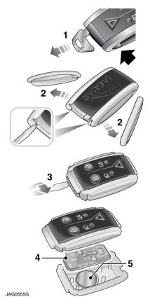
When the battery needs renewing there will be a significant decrease in the effective range of the key transmitter and the message **SMART KEY BATTERY LOW** is displayed on the message centre.
