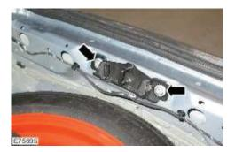
6. Loosen the liftgate to hinge Torx bolts.
