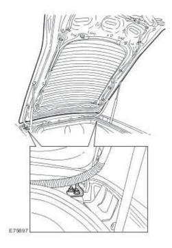
10. With the liftgate closed, check the alignment of the liftgate to the roof panel and bodyside panel. The liftgate should be central in its aperture.
