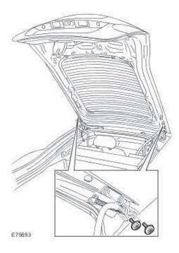
7. With the liftgate closed, check the alignment of the liftgate to the roof panel. Profile of the liftgate to roof panel should be 2 mm below flush.
