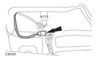
${f 3.}$  Disconnect the luggage compartment lid release switch electrical connector.
