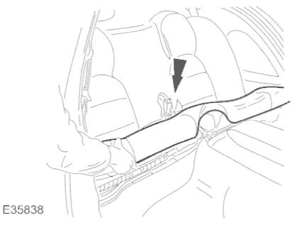
3. Raise seat cushion for access, pass seat belt anchors through central penetration and remove seat cushion from vehicle.
