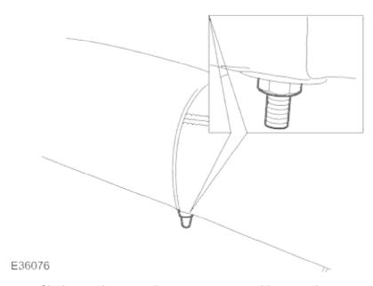
2. Slacken and remove the two rear seat cushion securing nuts.
