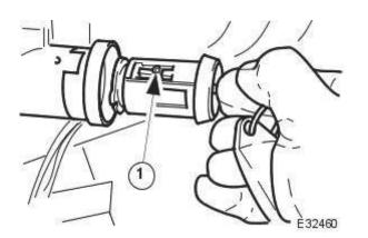
**3.** Install the lock barrel to the steering column lock.
