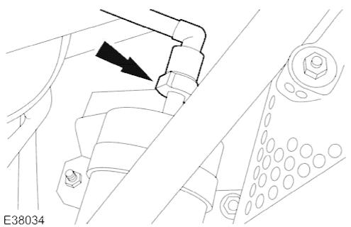
4. Disconnect the fuel tank to fuel filter fuel line. <<310-00>>
