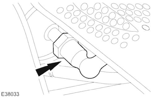
3. Disconnect the fuel filter to fuel injection supply manifold fuel line. <<310-00>>
