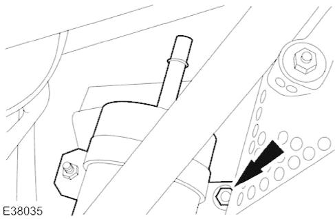
5. Remove the fuel filter and bracket.
