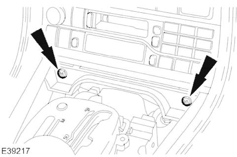
7. Slacken and remove the two forward securing bolts.
