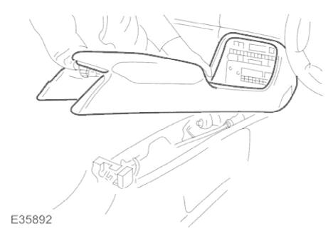
8. Position console for access, disconnect cigar lighter and valet switch harness multiplugs, lift console clear of 'J' gate and remove from vehicle.
