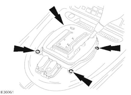
4. Slacken and remove the four center console veneer panel securing screws and remove the mounting plates.
