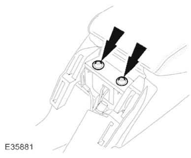
6. Remove console end trim cover and slacken and remove the two rear securing bolts.
