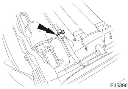
4. Disconnect harness multiplug from motor and sever and remove tiestrap securing harness to seat frame.
