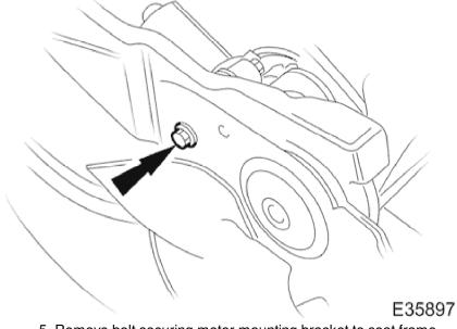
5. Remove bolt securing motor mounting bracket to seat frame.
