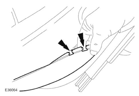
4. Withdraw the trim and 32 clips from seat back finisher and position trim for access.
