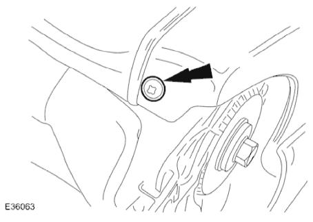
3. Slacken and remove the two screws securing the lower section of the seat back finisher to the frame.
