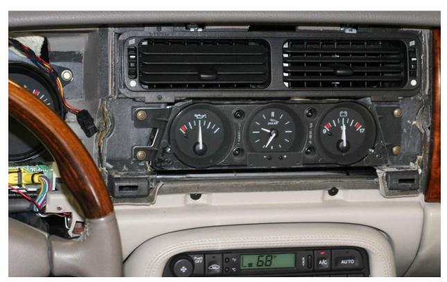
22. Using the screws removed from the navigation monitor, fasten the new gauge cluster to the dash.
