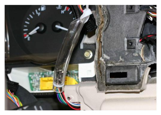
8. Clip the tie-wrap off of the clear tubing on the pulling tool and withdraw the tool from the wires. You may need to stagger the terminals in the clear tube to get them out without excessive force.Pull the longer red and black wires in the harness the rest of the way out from the cavity.
