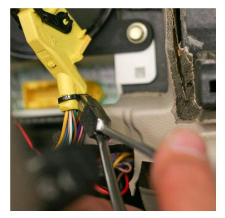
14. On each of the connectors, pry off the hood retainer gently with a pair of pliers.
