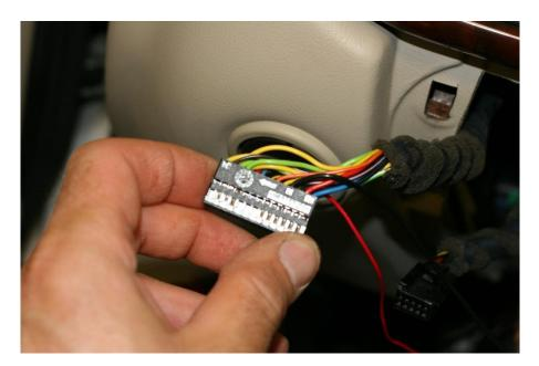
If you make a wiring error, a terminal can be extracted by gently pressing the tab in the window and pulling on the wire at the same time.
