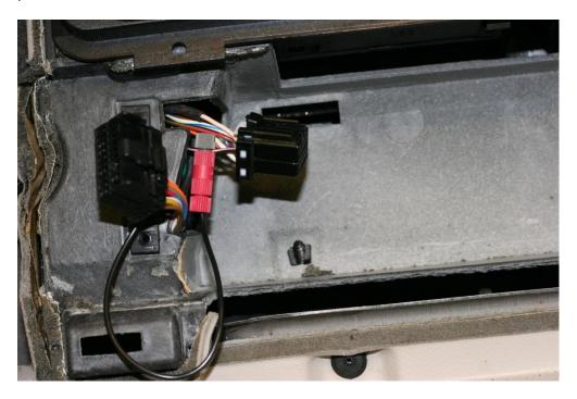
11. Locate the two main instrument panel connectors. One is yellow and the other is black.
