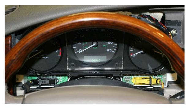
12. Release each of the connectors by depressing the tab-lock (pointed to in photo below) and pulling the hinged black plastic bail away from the wire end of the connector.
