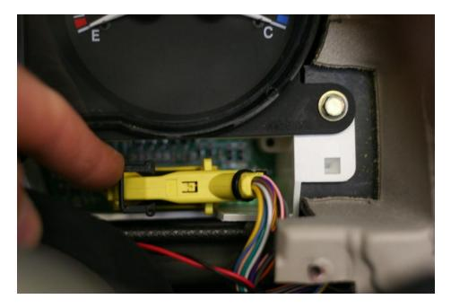
20. Tuck the black and red wires under the speedometer white plastic shell:
