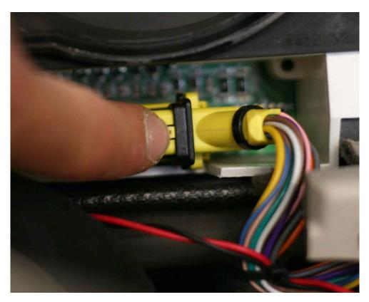
13. On each of the connectors clip off the zip tie at the harness with diagonal cutters. Be care not to damage the wires.
