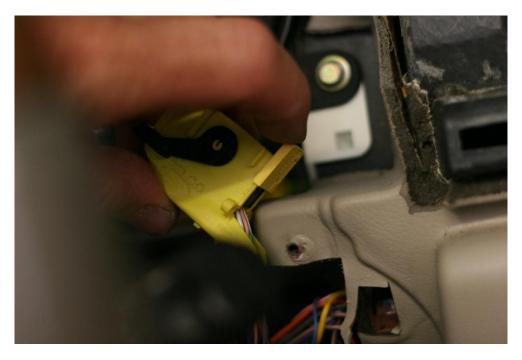
18. Replace the tie wraps on the hood retainers. Add another tie wrap to tie wrap to fasten the new harness to the existing one.
