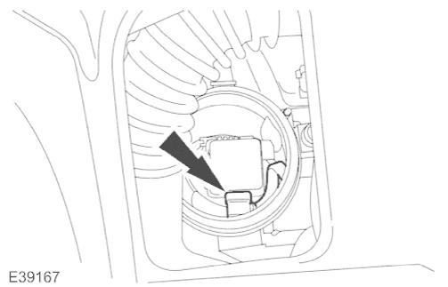
3. Disconnect the low beam headlamp bulb electrical connector.
