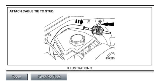
15. Attach the new filter, and then cable tie the assembly to the hose and attach the cable tie to the stud (Illustration 3).
