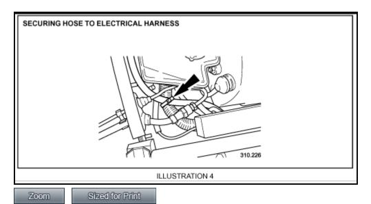
16. Secure the hose to the electrical harness using a cable tie and cut the protruding tail (Illustration 4).
