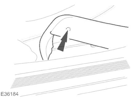
3. Release cover trim securing clip from brake lever and remove cover trim.
