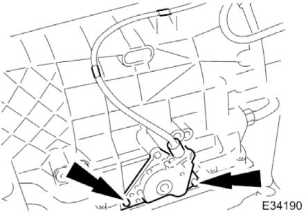
5. Remove the rotary switch retaining fixings.
