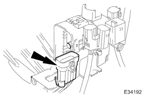
3. From above, disconnect the rotary switch harness multiplug.
