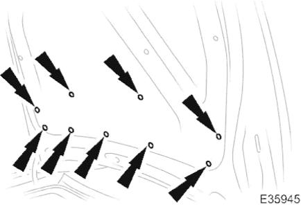
1. With trunk lid fully open, remove and discard fasteners securing liner to forward edge of lid.
