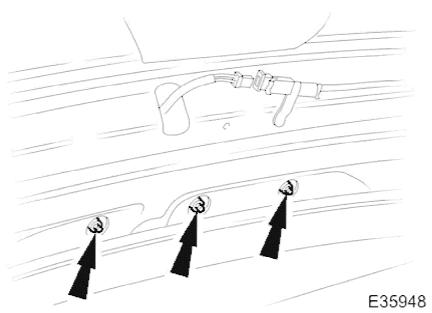
4. Remove three nuts securing stop lamp to trunk lid.
