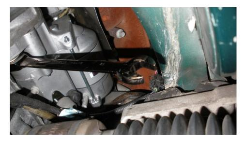
10. Now the starter is loose and can be removed at the steering rack along, down. You have to push the starter upwards-back and turn it, to get it out. This part is a little tricky and was complicated.
