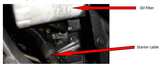
6. According to JTIS: Now loosen the cable to the starter.
