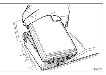
A second fuse box is situated within the bulkhead extension on the passenger's side.
