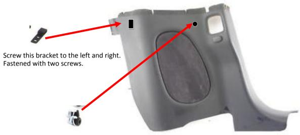
Screw this bracket to the left and right. For this you have to drill a hole in the Rear Quarter Trim Panel. Hold the bracket from behind with a nut.
