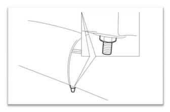
2. Raise seat cushion for access, pass seat belt anchors through central penetration and remove seat cushion from vehicle.
