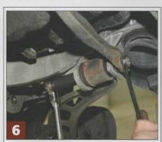
The forward lower bush has a conventional 18mm bolt and 22mm nut with no provision for adjustment. Note the position of the spacer between the alloy subframe and the steel bracebar
