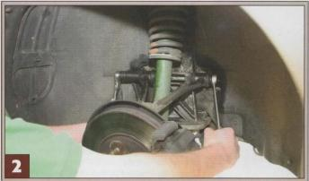
Before starting to dismantle, give the entire shaft and bush assembly a good soaking with penetrating oil. Then use a 24mm AF socket and spanner to loosen the main shaft. Note the special chrome plated shaped washers, they are positioned both sides of each bush and need to be retained even though they may look to be part of the old bush
