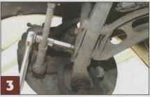
A pair of sandwich plates tie the two parts of the lower control arm to the spring/damper assembly, effectively taking the entire weight of the front of the car. Remove the two T60 Torx headed bolts - heat the threaded portion of the forward part if necessary to loosen. The suspension assembly should then drop free of the spring/damper
