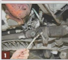
The first task is to undo the four 13mm bolts securing the steering rack to the subframe, as the rack ends and gaiters block the exit path of the lower rear securing bolt. It's not necessary to touch the hydraulic connections or even loosen the steering column, just ease the rack away and tilt it so that the lower control arm bolts can be removed
