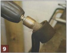
In many cases there will be corrosion in the arm itself. Within reasonable limits the rust can be cleaned away with a wire brush or finishing paper, but if doing this opens up the hole so far that the new bush remains loose, a new arm will be needed
