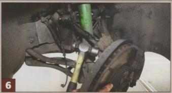
Use a punch or other slim bar to hold the arm loosely in place while the 18mm upper balljoint nut is undone (right). Then, with the nut still loosely on by a couple of threads, shock the housing (above) to release the taper; it will normally take several sharp hits. While the arm is removed be sure to support the hub assembly sufficiently to prevent damage to the lower balljoint
