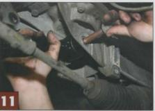
Reassembly is a reversal of the stripdown procedure, but with three important points to remember. Coat both the lower bush and drop link bolts with copper grease to prevent seizure in the future. Clean the T60 Torx bolts thoroughly and recoat with Loctite or similar. Only tighten the lower bush and drop link bolts with the weight of the car on the suspension, otherwise the bushes will remain permanently twisted, leading to premature failure
