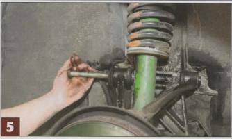
Then, as the shaft slides fully out of the sub frame, recover the forward shims and washers. Note that what appears to be a washer is in fact part of the collapsed bush, in many cases the entire bush has worn so far it can simply be twisted out of the control arm
