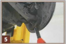
With the arm still located in the subframe, loosen the 19mm lower balljoint nut, leaving it on by just a couple of threads. The arm can then be manoeuvred out of the subframe and swivelled round to gain sufficient access for the hammer blows necessary to release the taper. If only changing the bush be very careful not to cause damage to the balljoint gaiter
