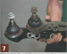
While technically available as a separate item, removing and replacing a lower balljoint successfully requires the skills and equipment of a professional engineer, and so it is almost always more practical to fit a completely new arm, especially if both the balljoint and bush are unserviceable
