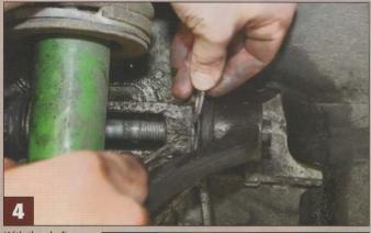
With the shaft halfway out, gently lever the rear arm and bush away from the subframe turret and recover any shims, together with the inner shaped washer
