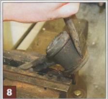
If the old bush refuses to come out easily, lock the arm in a vice and drive the bush out with a cold chisel. As can be seen below, over time the bearing material wears away and the sleeve then rusts, locking the two together and in turn causing the whole lot to turn in the arm
