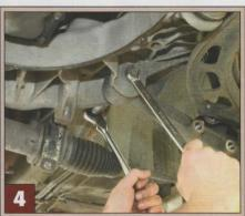
From VIN 031302, the 18mm bolt (and 22mm nut) securing the lower rear bush has an offset shank used to move the arm in or out slightly during camber adjustment - earlier cars may have had these bolts retro-fitted. The offset bolt can be identified by a raised strip on the bolt head flange (see below), the direction of which should be noted prior to disassembly
