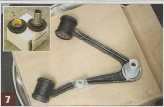
If the balljoint is still serviceable with its gaiter in place and untorn, replace only the bushes. If the ball joint is unserviceable a new control arm will be needed which will come with the bushes already fitted. Note that the bush is more like a bearing than a conventional rubber item and it is identical to those used on the XJ-S and XJ saloons prior to the 4.0-litre XJ40
