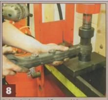
Both bushes have steel flanges, which unfortunately allow nowhere to support the arm while pressing them out. While the rear bush can be removed with just two sides of the arm exposed, it is much safer to chisel/hacksaw the entire flange off (below) and then use a suitable section of pipe to press against
