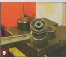
When fitting new bushes the correct Jaguar tool (shown in background) is essential to prevent damage to the rubber face. Position the new bush, flange facing forward in the arm, sit the specially shaped tool on top, and place the whole lot in the press, pushing the bush in until it seats fully
