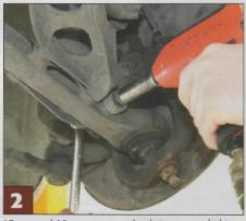
13mm and 15mm spanners/sockets are needed to unbolt the anti-roll bar vertical link. If either of the link bushes are torn/perished, fit a new pair of links
