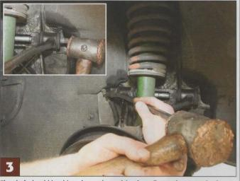
The shaft should be driven forwards, applying force first to the protective lug at the end of the thread and then via a chisel or lever to the back of the bolt head
