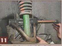
To reassemble, first coat the shaft well with copper grease, then assemble the various washers and shims around the forward bush, hold it up and feed the shaft through. With the arm supported, the washers and shims can then be positioned around the rear bush and the bolt slid fully home. As the bearing within each bush allows movement, the upper bush shaft can be tightened fully without weight on the suspension
