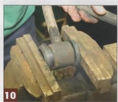
No special tools are needed for these bushes: just use the vice to push one half in, then fit the sleeve followed by the other half and push them fully in as well. Be sure to keep everything aligned correctly, however, as it is easy to damage the bearing material inside. If the halves seem not to seat fully, don't worry, they will when fitted and tightened
