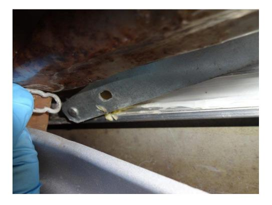
Next you need to lever out the arms from the plastic clips, I used a small prise bar.
