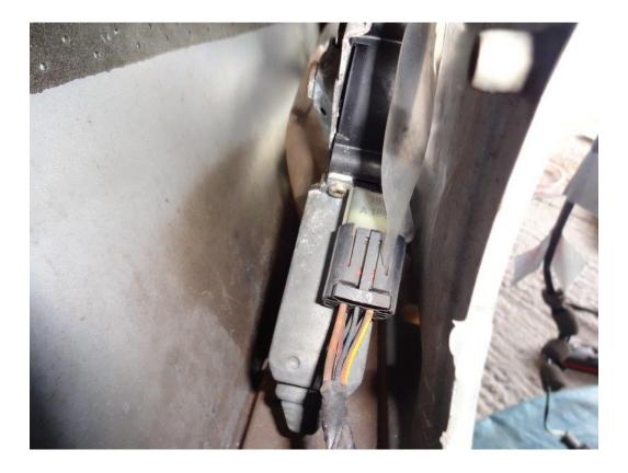
Release the locking tab by pushing here.
