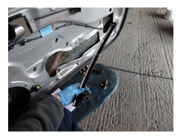
Lower the glass and then remove the screw holding the retaining bracket.
