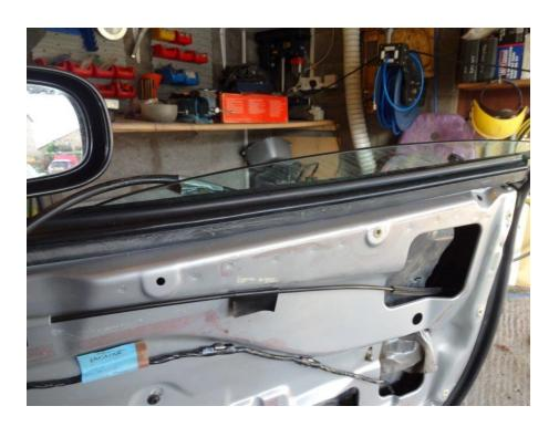
Next you have to remove the retaining clips from two of these on the bottom rail of the regulator. It's worth buying a couple of new clips in advance as the old clips may break.
