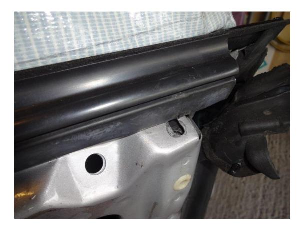
...and then the two torx screws from the bottom runner adjuster.
