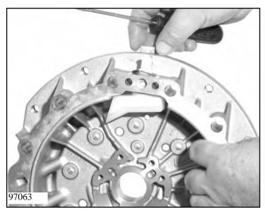
Take off the cover from the breather. Remove the breather's locking disc and push out the breather and the O-ring.
