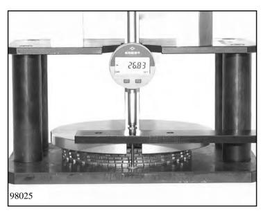
Determine thickness  $\mathbf{M_E}$  of the brake E clutch pack according to
