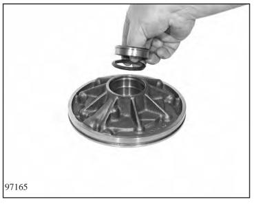
Complete pump 10.010. First put sealing ring 10.010/140 into the pump housing and press in the needle bearing 10.010/150 with assembly drift 5x46 000 954 in the mandrel press.
