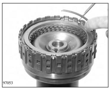
Take out the snap ring for clutch A and remove its complete clutch pack.
