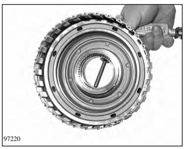
Cover one of the two oil supply bores and press out the piston with compressed air. Remove three O-rings from piston B.
