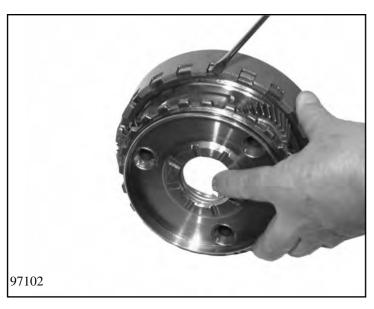
Place a new O-ring 32.290 on planet carrier I 32.100. Insert the planet carrier into ring gear II 32.120, and secure it with snap ring 32.130.
