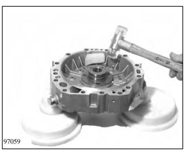
Loosen 10 machine screws (countersunk); two opposing machine screws should not be unscrewed all the way. Drive out the pump by striking these two screws carefully with a plastic-faced hammer.
