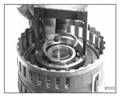
Turn over cylinder DE by  $180^{\circ}$ . Put two O-rings (73.010/152 and 73.010/154) on piston D 73.010/150 and press it into the cylinder.
