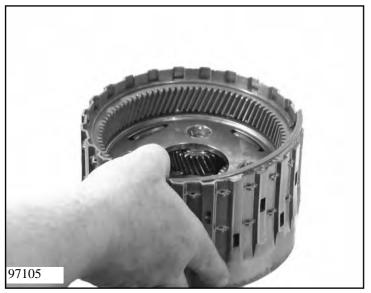
Insert ring gear III 32.240 with the outer engaging gears towards the top and secure it with snap ring 32.250. To put the snap ring in position, lift ring gear I slightly.
