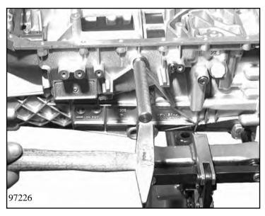
Install shaft seal 01.010/120 into the transmission housing using the drift 5x46 001 261.
