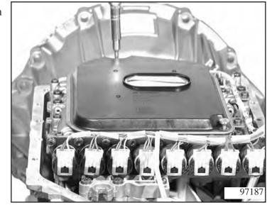
Use grease (petroleum jelly) to attach and align seal 03.030 to the transmission housing.
