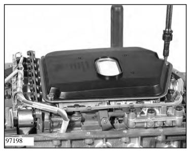
Remove the filter and the O-ring by unscrewing the 2 machine screws.
