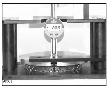
Determine thickness  $\mathbf{M}_{\mathbf{D}}$  of the brake D clutch pack according to
