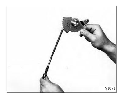
Insert the detent disc and connector rod into the transmission housing and push selector shaft 01.010/130 through the detent disc.
