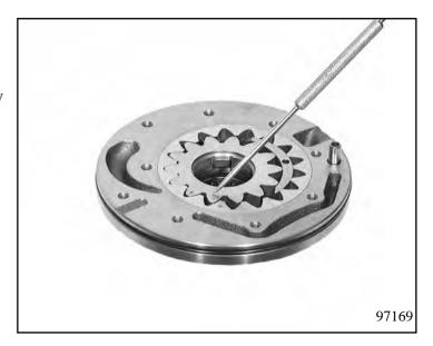
Put two rectangular-section rings 10.020/140 on stator shaft 10.020/120. In order to be able to mount the stator shaft on the intermediate plate, the two parts have to be positioned together properly. The procedure for doing this is described on the next page.
