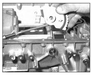
Now the detent disc and the connecting rod can be taken out. Lift off the shaft seal using a screwdriver.
