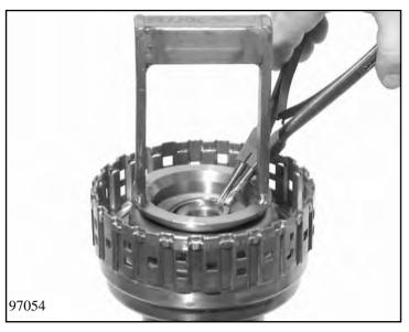
Using assembly bracket 5x46 001 499, press down the oil dam and remove the snap ring with suitable pliers. Take out the oil dam and cup spring, and pull the O-ring off the oil dam.
