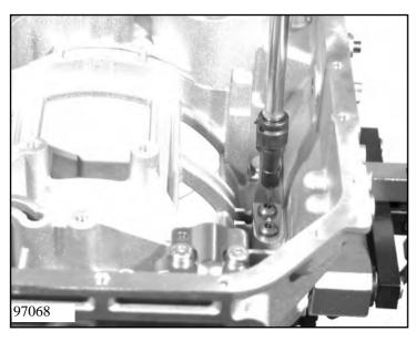
The detent spring normally remains in the transmission housing. If it is to be removed, unscrew the two Torx screws.
