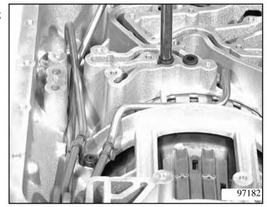
Screw testing plate 5p01 003 040 onto the control unit connection on the housing and check the function of all clutches/brakes by applying compressed air to the marked bores.
