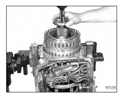
Turn the transmission 180° and loosen the 10 hexagonal screws.
