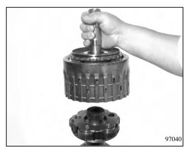
Disassemble planetary drive III by taking the sun wheel shaft out of planet carrier III.
