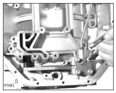
Press the pawl down, and fasten guiding plate 01.070 with four Torx screws 01.080.
