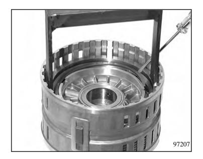
Turn over cylinder D/E, take out the brake E snap ring, and remove the complete clutch pack.
