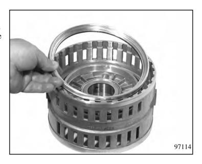
Insert cup spring D 73.010/160. Using assembly bracket 5x46 001 501, press down cup spring D in the mandrel press and secure it with snap ring 73.101/170 (flat side upwards).
