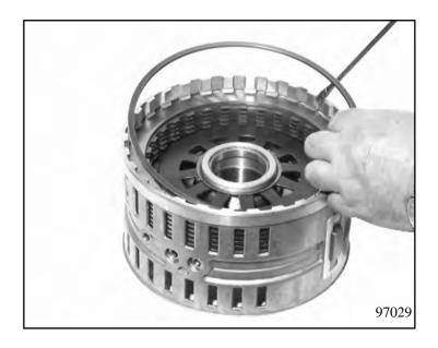
Using assembly bracket 5x46 001 502, press down cup spring E in the mandrel press, take out the split stop ring, and remove the cup spring.
