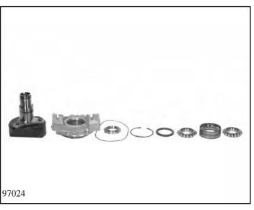
Take out the snap ring with pliers and lift the extension off the output flange. Then lever out the shaft seal using a suitable screwdriver and push out the ball bearing in the mandrel press. If necessary, heat up the extension to approx. 70° C using a fan heater or similar device.
