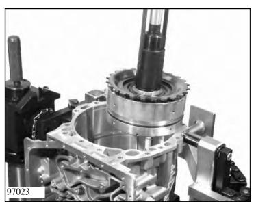
Turn the transmission by 90° and insert lifting device 5x46 000 831 into cylinder F by lifting the bracket handle. Releasing the bracket handle locks the device. Turn the device until it latches into place.
