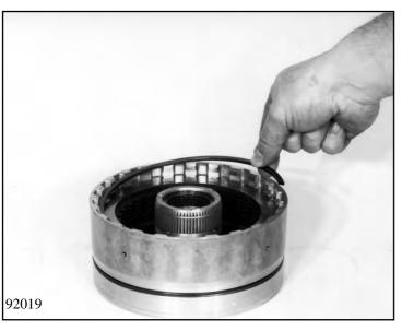
Take out the snap ring and lift out the complete clutch pack of brake F.
