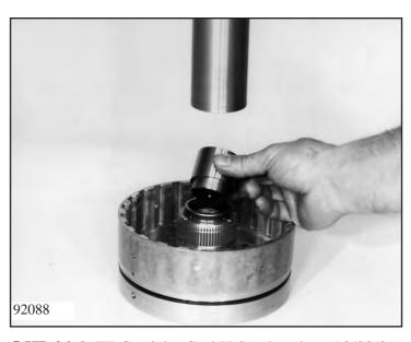
Put O-ring 75.140 on cylinder F 75.010. Press needle roller bearing 75.020 into cylinder F with press-in fixture 5x46 001 006 in the mandrel press, and secure it with snap ring 75.030.
