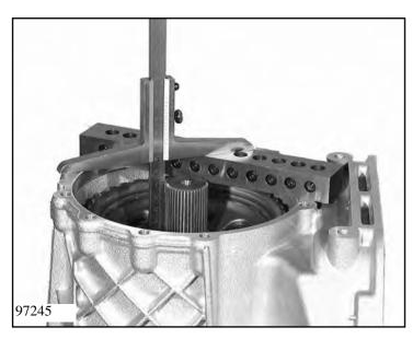
Using a depth gauge and a measuring bar, determine distance **B** between the machined face of the transmission housing and the machined face of the parking lock wheel.
