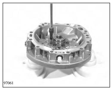
Unscrew 5 countersunk screws, warm up the housing around the stator shaft to approx. 70° C and drive the stator shaft out of the intermediate plate using the plastic-faced hammer.
