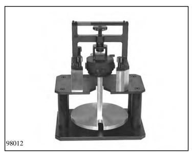
Fasten adjusting device with 4 knurled screws to the measuring fixture using the intermediate pieces.
