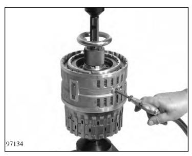
Screw lifting device 5x46 001 077 (fastened together with adapter 5w46 000 003) into tower I.
