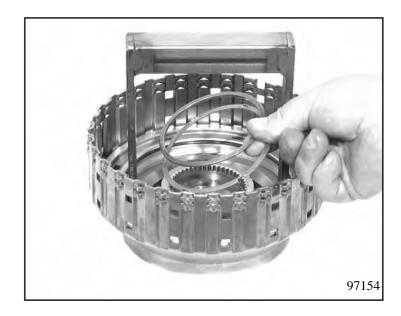
Insert the complete clutch pack B. Begin with spring clutch disc 72.082 followed alternatingly by outer clutch disc 72.090 and lined clutch disc 72.100. Secure the top outer clutch disc 72.110 with snap ring 72.130.
