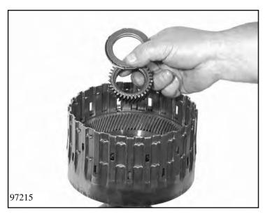
Take out the axial needle roller bearing and sun wheel.
