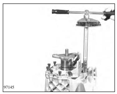
Put on the output assembly and fasten it with 10 hexagonal screws 14.070. Turn the housing 180°. Remove assembly fixture 5x46 001 077.
