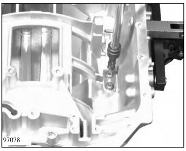
Attach the 01.010/180 detent spring with two 01.010/200 Torx screws but do not tighten them, so that the detent spring can still slide easily.
