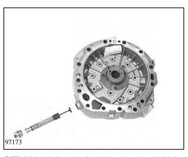
Insert the flow control valve (consisting of piston 10.020/150, pressure spring 10.020/160, sleeve 10.020/170) into the intermediate plate and secure it with screw plug 10.020/180.
