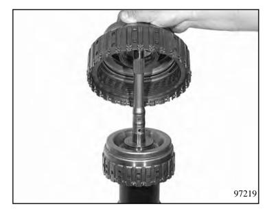
**Note!** The input shaft is meshed with clutch B.
