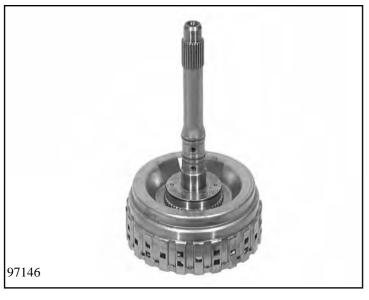
Place a new O-ring 70.014 and two rectangular-section rings 72.140 on cylinder A 70.010 with the input shaft.
