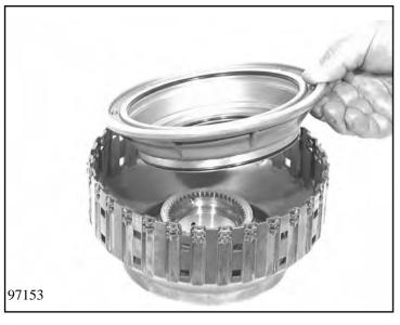
Put two O-rings (72.030, 72.040) and sealing ring 72.050 on piston B 72.010. Press piston B into cylinder B.
