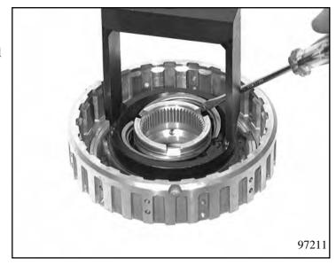
Carefully press out piston C using compressed-air via the oil feed bore. When doing this, block the other two bores.
