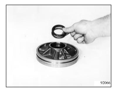
Press out the sealing ring with the needle roller bearing in the mandrel press. The diameter of the pressure bolt should be approx. 42 mm.
