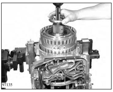
Align the bores for the oil pipes. Using a crane, carefully insert tower I into the transmission housing.
