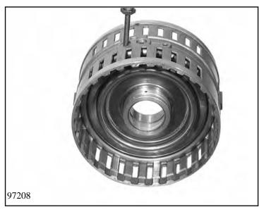
Apply the compressed-air gun to the oil feed bore and force out pistons D and E with compressed air.
