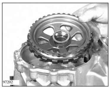
Take out the shim and the parking lock wheel of the transmission housing.
