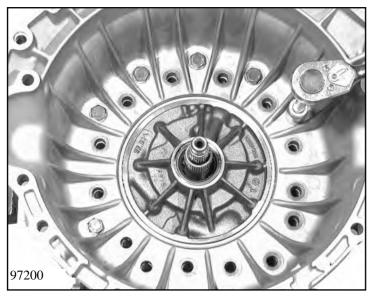
Put converter bell housing 22.010 onto the intermediate plate so that 20 hexagonal screws can be screwed in as follows:
