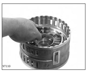
Complete cylinder DE 73.010/110. First put on two O-rings (74.010/140, 74.010/150) to the bushing 74.010/130 and press it into cylinder DE. Drive two shaft keys 73.010/140 onto the center of cylinder DE using the plastic hammer.
