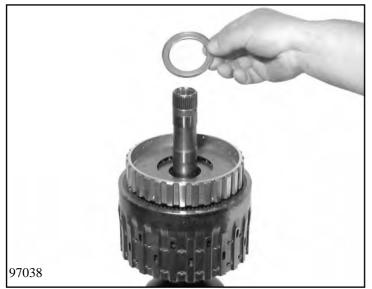
Lift off the needle roller bearing.
