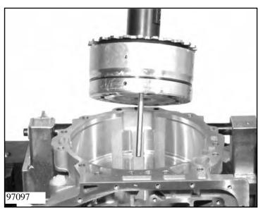
Turn the transmission housing by 90°. Insert the complete unit so that the dowel pin can be led into the top hole in the center of the transmission housing.
