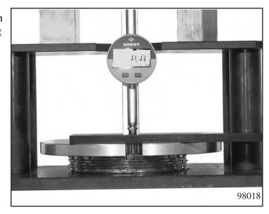
Now measure down to the base plate using the measuring bar.
