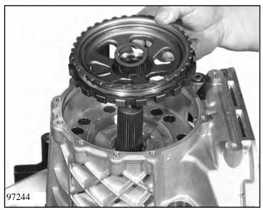
Turn the transmission 180°. Put in parking lock wheel 24.040, and place shim 14.080 on top of it.
