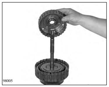
Align the discs for clutches A and B, and insert intermediate shaft 72.160, turning it as you put it in.
