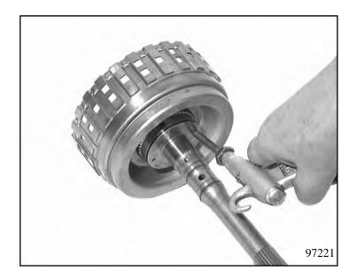
Take off the O-ring and the two rectangular-section rings from the drive shaft.
