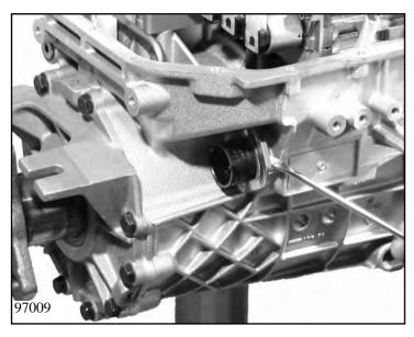
Disconnect the transport protection cap from the wiring harness socket, unlock the retaining clip using a suitable screwdriver, and press the socket into the housing by hand.
