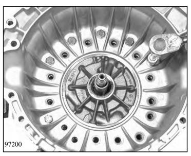
If only the converter bell housing is to be removed (damage!) unscrew the six remaining hexagonal screws and separate the converter bell housing from the intermediate plate. The intermediate plate remains on the transmission housing.
