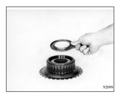
Insert the complete freewheel into brake F, turning it as you put it in. Now insert snap ring 77.130 using assembly tool 5x46 000 892 (or by hand).
