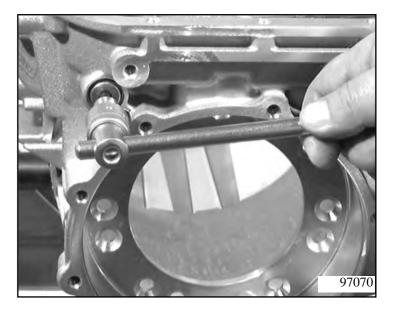
Lever out the bolt of the transmission housing. Now the pawl and spring can be removed.
