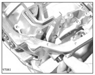
Insert pawl 01.040 and leg spring 01.050 into the transmission housing and fix it in place by pressing in bolt 01.020. Then plug up the bore using a screw plug with seal 01.090.
