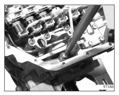
Put O-ring 27.460 on the stub pipes from filter 27.450. Fasten the filter with two machine screws 27.470.
