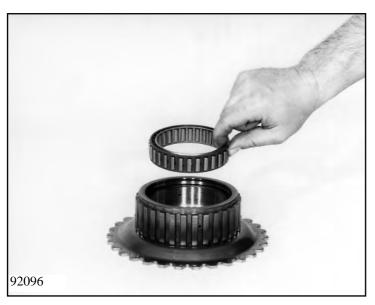
Insert the freewheel cage (with the collar at the top) into the freewheel outer race.
