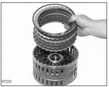
Turnover cylinder DE and insert complete clutch pack E beginning with outer disc 74.050 followed alternately by clutch lined disc 74.060 and outer disc. Secure top outer disc 74.070 with snap ring 74.090.
