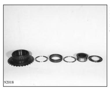
Remove the snap ring and disassemble the complete freewheel down to the following parts: fixing washer, inner sprag race, cover disc, freewheel cage, cover disc, and outer sprag race.
