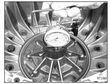
Determine axial play by pressing and pulling on the handle (repeat measurement several times)
