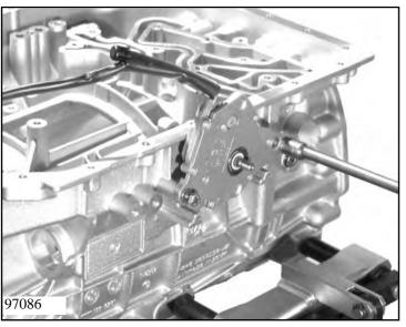
Put the 01.480 switch on the selector shaft and tighten it with two hexagonal screws (01.590 and 01.620) on to the transmission housing.
