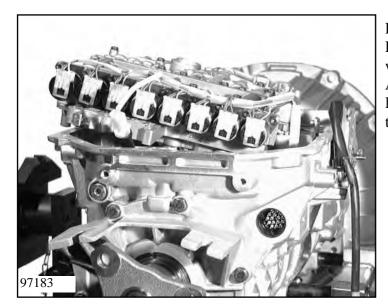
Put the control unit on loosely. Put two new O-rings 27.260/116 on the wiring harness socket outlet. Align the socket outlet so that the two lugs on the socket outlet can engage in the lug on the transmission housing.
