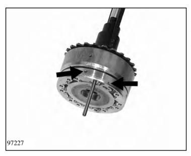
Screw the fitting pin (an M8 bolt with its head cut off) into the single threaded bore between the oil feed and the lubricating oil feed.
