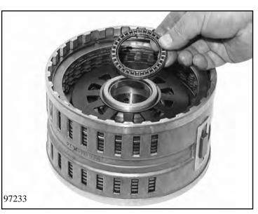
Lubricate axial needle roller bearing 32.340/120 with petroleum jelly and attach it to the cylinder ridge 73.010/110 (on the brake E side).
