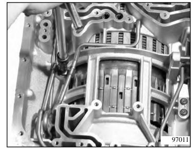
Release the two retaining rings for locking the pressure springs and remove them both.
