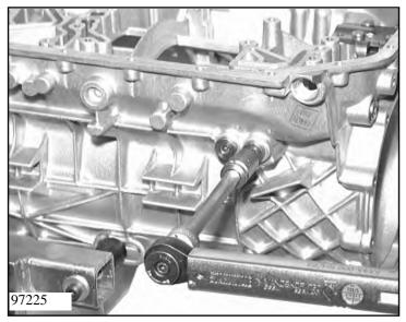
Screw new screw plugs 1x 01.650 and 2x 01.210 into the transmission housing. Insert transport plugs 01.230 and 01.240 hand-tight.
