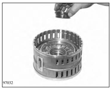
Force the bushing out of cylinder D/E. Remove the two O-rings from the bushing.
