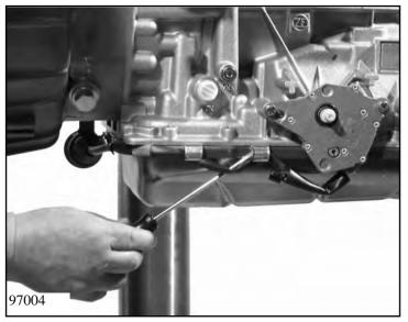
Use a screwdriver to lift out the wiring harness at the cable clamps.
