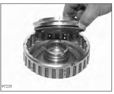
Mount new O-rings (75.010/130 and 75.010/140) on piston C 75.010/120. Press the piston into cylinder C 75.010/110.
