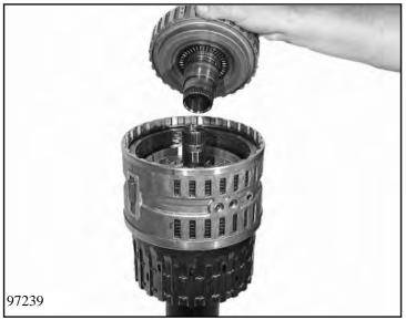
Attach axial needle roller bearing 31.090 to cylinder C on the sun wheel shaft side. Put clutch C into brake D, turning it backwards and forwards until the clutch pack fully mesh with the gears.
