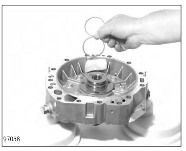
Place the complete oil supply on suitable supports. Take off the two rectangular-section rings from the stator shaft.
