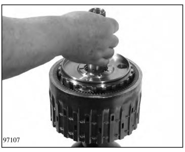
Turn the planetary drive as you put it on the planet carrier.
