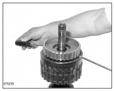
Using two screwdrivers, lift up planet carrier E and take off the thrust washer.
