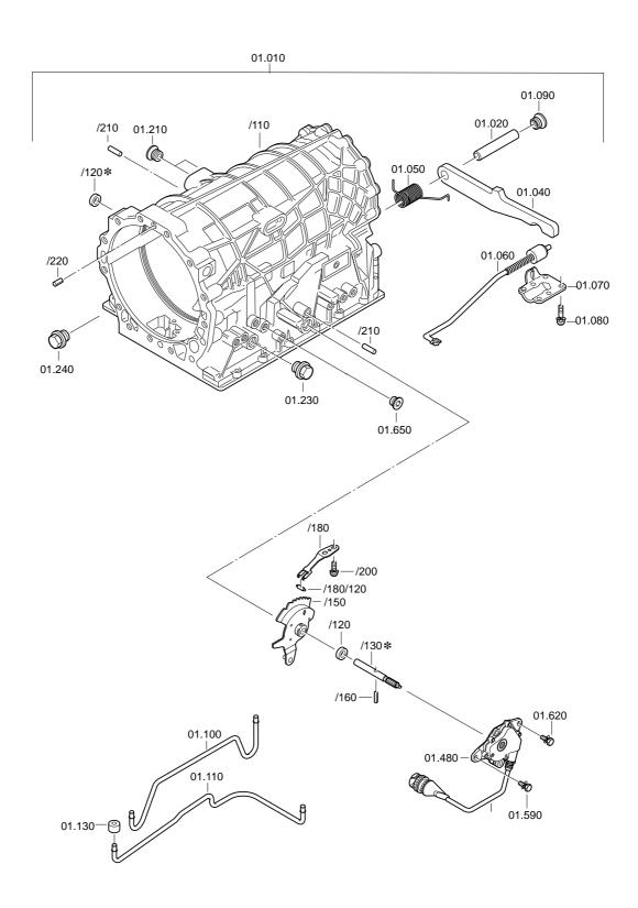
Drive the plug 01.130 into transmission housing 01.010/110 by using the tool 5x46 001 135.
