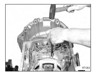
Using a suitable tool, drive in two sealing bushes 01.350 between the transmission housing and cylinder DE.
