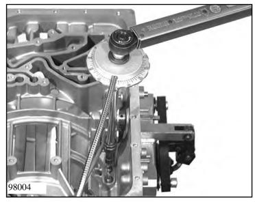
Align the detent spring's roller on the center of the detent disc, and screw it tight with helping tool 5w04 000 583 in this position.
