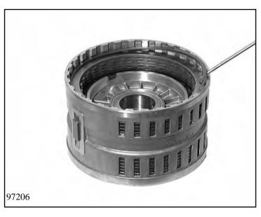
Unsnap the snap ring from brake D and take out the complete clutch pack.
