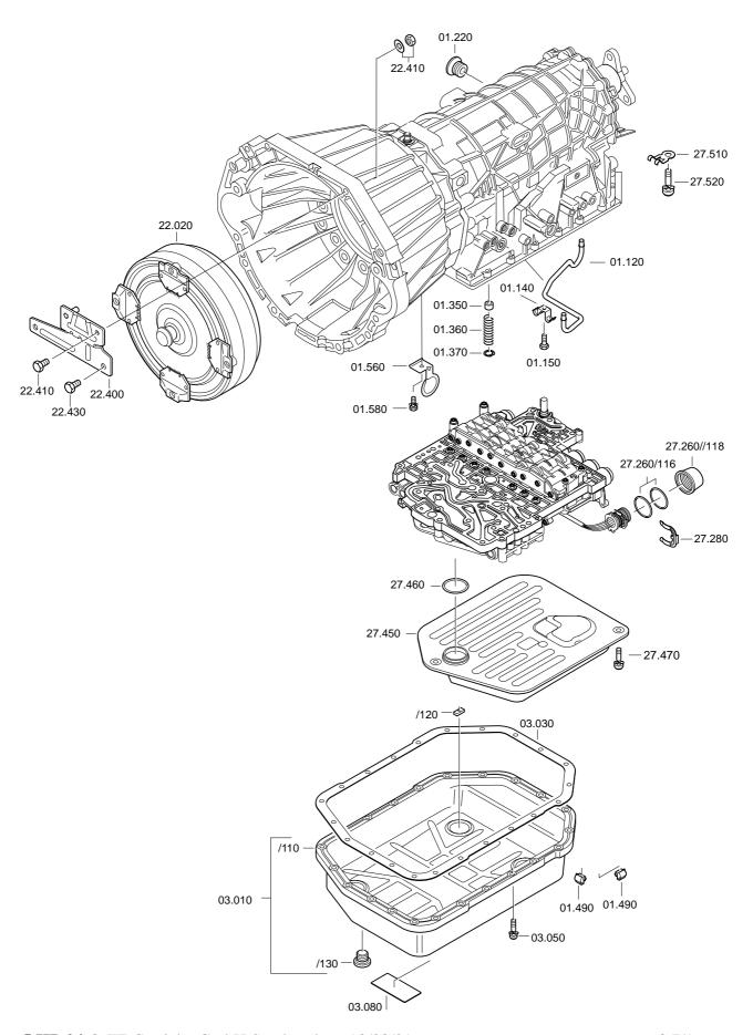
Turn the housing 90°. Mount the remaining oil pipe (01.120) into the cylinder E bore and the transmission housing using driving tool 5x46 001 534. Attach with retainer 01.140 and
