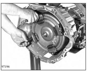
Remove the converter bracket and remove the converter using two extractor handles 5x56 000 090.
