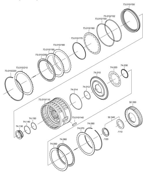
Press disc carrier E 32.330 on to the planetary drive.
