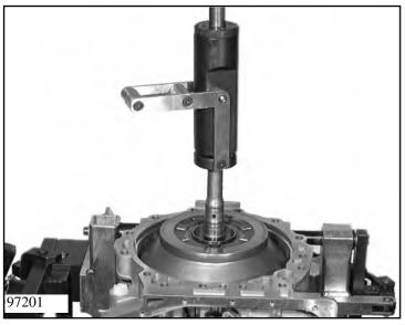
Take off the shim and the axial needle roller bearing.
