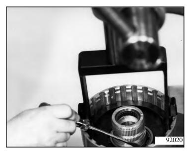
Push cylinder F out using two plastic punches.
