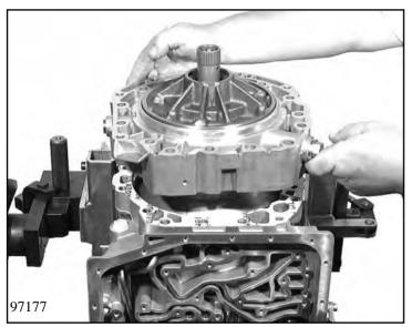
Coat the rectangular-section rings on the drive shaft with some petroleum jelly. Put the intermediate plate carefully onto the transmission housing and align it.
