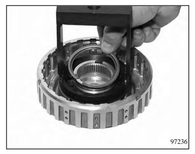
Put in complete clutch pack C beginning with spring clutch disc 75.010/170. This is followed by outer clutch disc 75.010/180 and lined clutch disc 75.010/190. Secure the top outer clutch disc 75.010/200 with snap ring 75.010/210.
