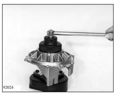
Unlock the slotted nut using a suitable chisel and loosen it with slotted nut wrench 5x46 000 787.
