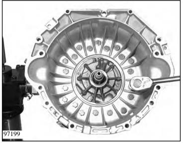
Turn the transmission 90° and remove the converter bell housing. Normally, it should be removed together with the intermediate plate. To do this, loosen and remove the 14 hexagonal screws. Pull off the gasket.
