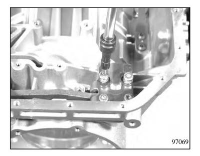
Remove the screw plug and sealing ring.
