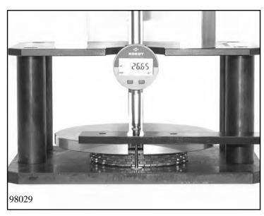
Determine thickness  $\mathbf{M}_{\mathbf{A}}$  of the clutch A clutch pack according to
