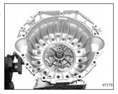
Clamp the measuring sleeve for device 5p01 001 415 on to the stator shaft using the three fastening screws, no play allowed.
