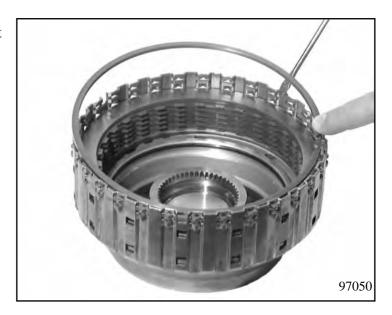
Press down the cup spring in the mandrel press using assembly bracket 5x46 001 500. Remove the snap ring with suitable pliers. Take out the fixing washer and the cup spring.
