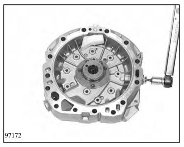
Mount breather 10.020/190 (with a new O-ring 10.020/200) into the intermediate plate and secure it with retaining disc 10.020/210.
