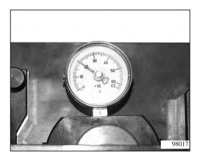
Then put measuring bar 5p01 060 330 on the measuring plate, insert the measuring base of the dial gauge into the groove of the measuring plate on the top plate of the pack and set the dial gauge to zero.
