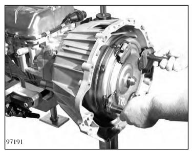
Screw in converter handles 5x56 000 090 and carefully insert converter 22.020.
