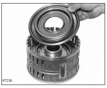
Turn cylinder DE over. Put new O-ring 74.012 on piston E 74.010 and O-ring 74.014 on the cylinder E. Press piston E into cylinder DE.
