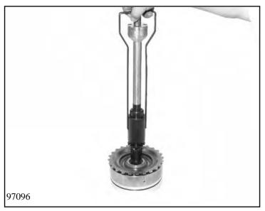
Insert lifting device 5x46 000 831 into brake F in such a way that the three raised areas on the cylinder hub engages into the recesses of the lifting device's collar.
