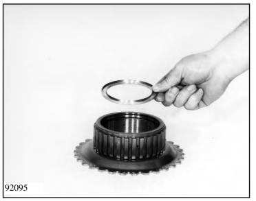
Complete first gear freewheel 77.120 by first pressing one of the freewheel's two covering washers completely into freewheel ring F.
