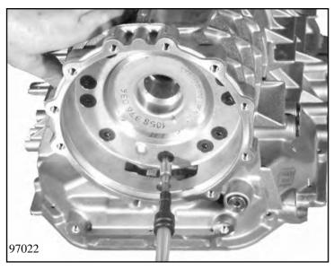
Turn the transmission 90° and unscrew the 12 countersunk screws used to secure cylinder F.
