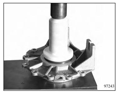
Put output flange 14.020 on counter support 5x46 000 946. Put the extension on the output flange. Place O-ring 14.060 on the extension.
