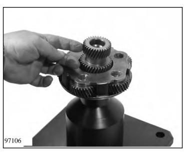
Take planetary drive (I and II with ring gear III) off the device. Put planet carrier III 42.010 onto the device and insert sun wheel 32.360.
