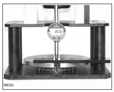
Determine thickness  $M_C$  of the clutch C clutch pack according to
