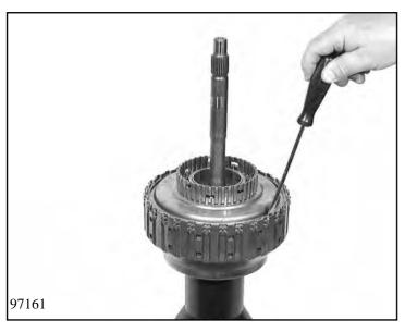
Put inner disc carrier C 72.190 into cylinder B and secure it with snap ring 72.200.
