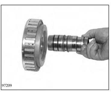
Press out the sun wheel shaft of the cylinder C using a suitable mandrel. Take the two O-rings and the two rectangular-section rings off the shaft.
