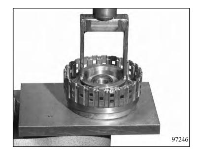
Insert the complete clutch pack A. Begin with spring clutch disc 70.090, followed alternately by outer clutch disc 70.100 and lined clutch disc 70.110.
