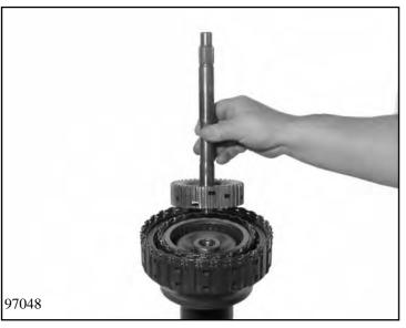
Lift up the intermediate shaft with inner disc carrier A. Remove axial needle bearing.
