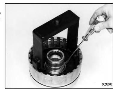
Insert the complete clutch pack, beginning with spring clutch disc 77.070. This is then followed by outer clutch disc 77.080 and lined clutch disc 77.090. Secure outer clutch disc 77.100 with snap ring 77.110.
