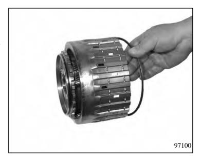
Insert sun wheel I 32.190 with the notch on the toothtip looking downwards. (Towards the output side to optimize the meshing sound.)
