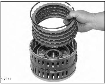
Insert the complete clutch pack D, beginning with spring clutch disc 73.010/180. This is followed by outer clutch disc 73.010/190 and lined clutch disc 73.010/200.
