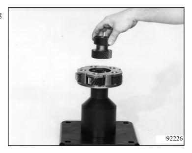
Put planetary drive I + II into device  $5x46\ 000\ 916$ . Take out the snap ring and remove ring gear III.
