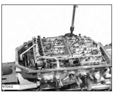
Loosen the inductive transmitter screw and remove together with holder.
