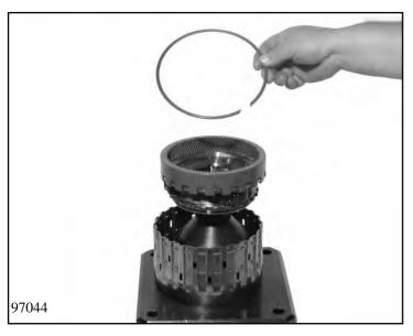
Take out the snap ring and separate planet carrier I and ring gear II from ring gear I.
