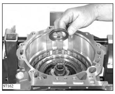
Place axial needle roller bearing 02.240 on tower I.
