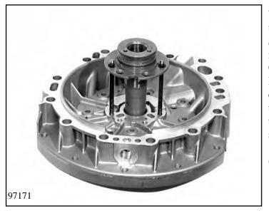
Warm the intermediate plate 10.020/110 up to 70° C using a hot-air blower. Screw two locating pins 5x46 001 007 into the intermediate plate. Guide in the stator shaft using the locating pins and secure it first with three countersunk screws 10.020/130. Remove the locating pins and screw in the rest of the countersunk screws.
