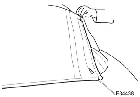
14. Using a piece of welding rod or similar draw wire, pull the outer tension cords through the headlining piping.
