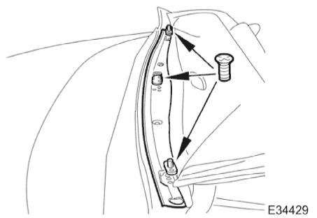
28. Position guide pins and latch striker and fit and tighten securing screws.
