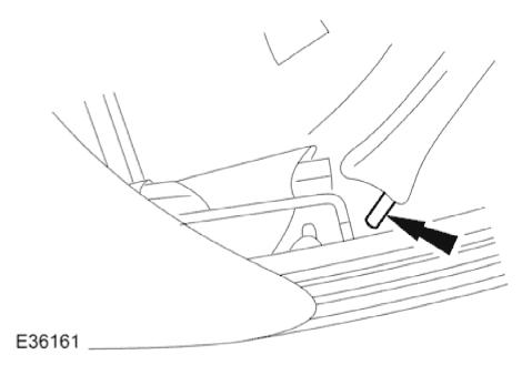
27. Position top cover and padding bag rearwards and release both headlining rear tension rods.
