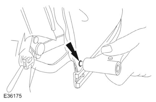
17. Align rear of headlining, pierce it through existing holes at riveting points in the retaining brackets and poprivet headlining to retaining brackets.
