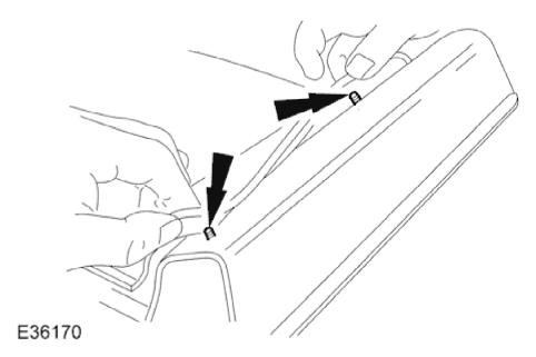
19. Fit and fully seat new fir tree fasteners securing headlining to frame.
