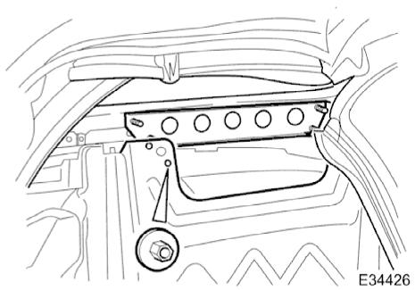
9. Slacken and remove squab panel stiffener bracket to body securing nuts and remove bracket.
