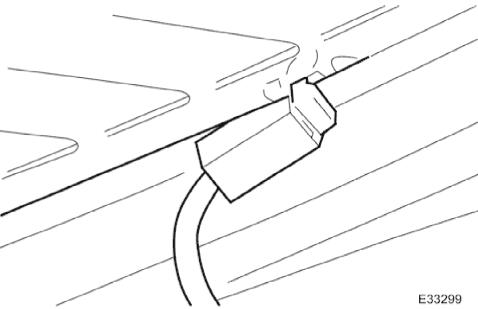
2. Disconnect heated backlight harness connectors and position harness clear of top.
