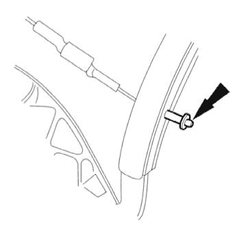
38. Release and remove tension cable retaining bushes, and disconnect cables from frame.
