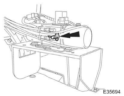
12. Position trunk RH liner for access and turn hydraulic pump valve fully counter-clockwise to manual operation position.
