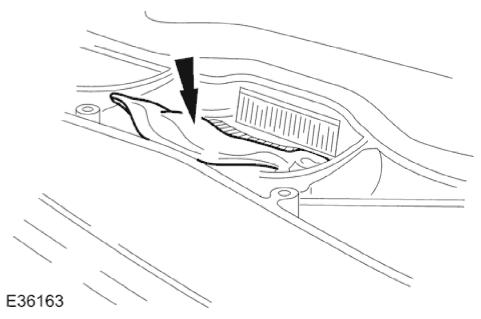
30. Release section of headlining secured by velcro strips to frame around pull-down handle aperture (bonded on early vehicles).
