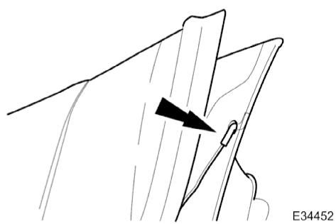
24. Using a piece of welding rod or similar draw wire, pull side tension cables through outer cover and secure them to frame.
