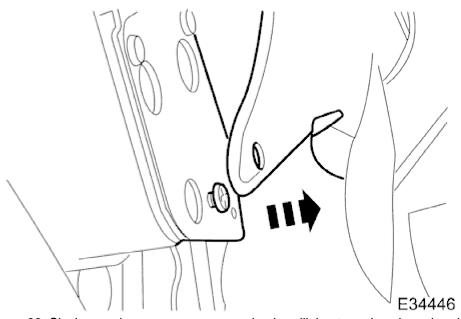
28. Slacken and remove screws securing headlining to main column bracket covers.
