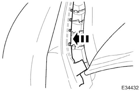
23. Release cover front retaining rod from retaining clips in frame and remove rod from cover.
