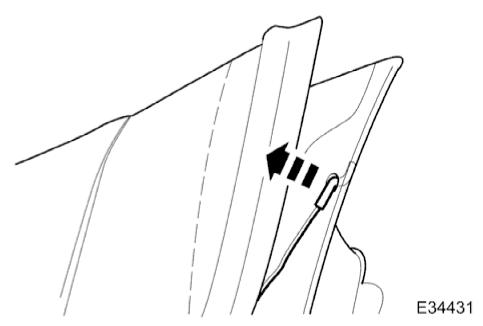
22. Disconnect roof side tension cables from frame.
