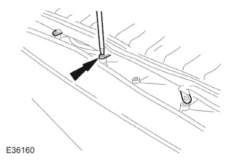
21. Align padding bag to frame and secure with 'P' clips and retaining screws.
