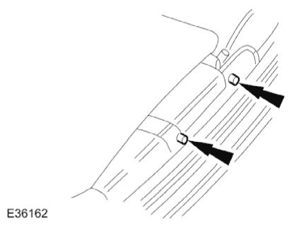
29. Drill out the two rivets each side, securing rear of headlining.
