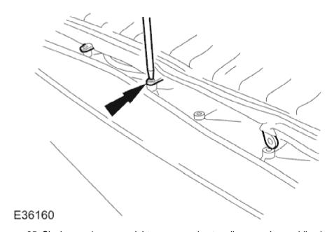
25. Slacken and remove eight screws and outer clips securing padding bag to frame.
