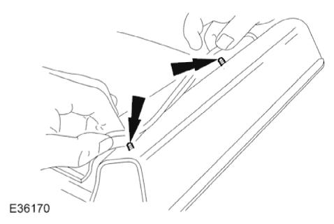
39. Release headlining fir tree or press stud fasteners from cantrails. Refer to Note in Step 42.
