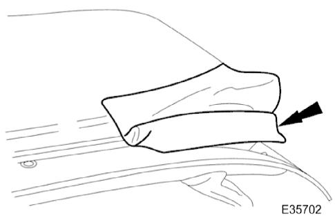
24. Noting the positions for installation, release bonded areas of padding bag from frame and withdraw bag from front of frame.
