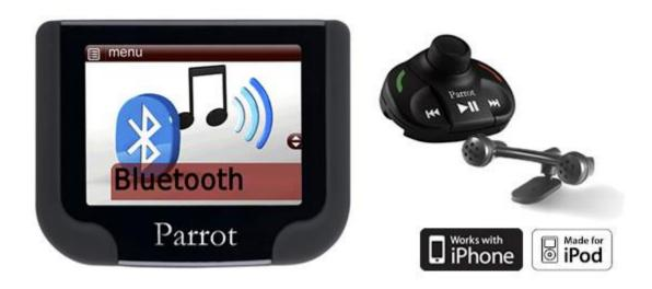
It is a Bluetooth hands-free system with a 2.4-inch high-resolution TFT color screen. A wireless remote control can be mounted on the steering wheel or dashboard and allows the driver to control all the functions of the MKi9200.
