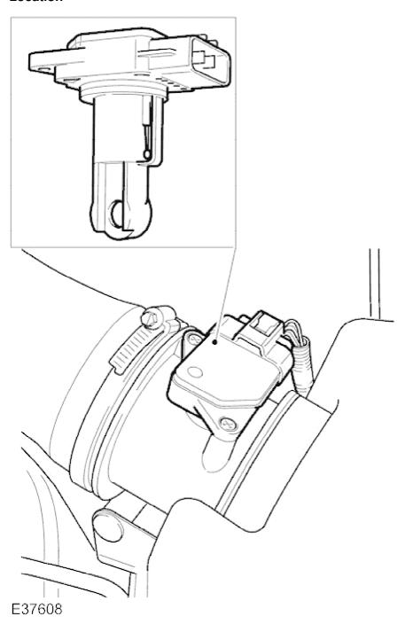
The MAF sensor informs the ECM of the rate of air flow entering the engine by producing a voltage which is proportional to the rate of air flow into the engine. The voltage produced by the MAF sensor increases as the rate of air flow increases. The ECM takes into account the density of the air entering the air intake system so that it is possible to maintain the required air to fuel ratio, and to compensate for variations in atmospheric pressure.
