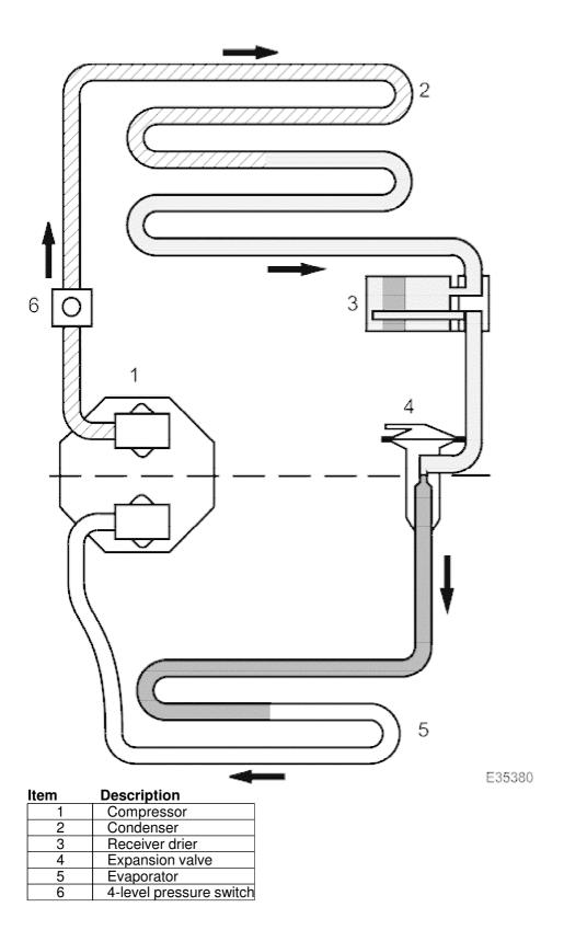
The Compressor draws low pressure, low temperature, refrigerant from the evaporator and, by compression, raises the refrigerant temperature and pressure. High pressure, hot, vaporized refrigerant enters the condenser, where it is cooled by the flow of ambient air. A change of state occurs as the refrigerant cools in the condenser and it becomes a reduced temperature, high pressure, liquid.
