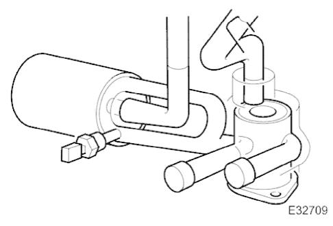
This valve is fitted between the oil pump outlet and the oil filter inlet.
