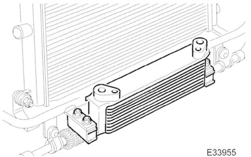
The engine oil cooler is located in front of the radiator, mounted off-center with two steady brackets bolted onto the front upper crossmember in front of the cooling module.
