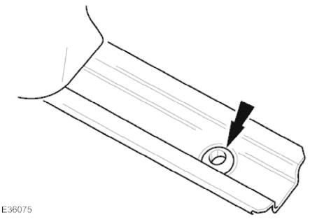
5. Slacken and remove the two seat rear securing bolts.
