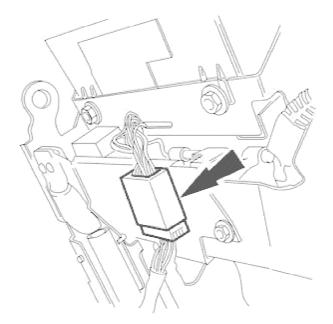
6. Position front seat for access, disconnect seat harness multiplug and remove seat from vehicle.
