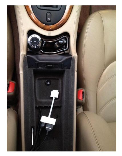
With everything in place you should be able to switch the ignition on and test everything. When the switch is in the center position, the stock nav system should be visible and when in position #2 the HDMI input should be in use. Position #1 is still available for another input if you should decide to add one in the future.
