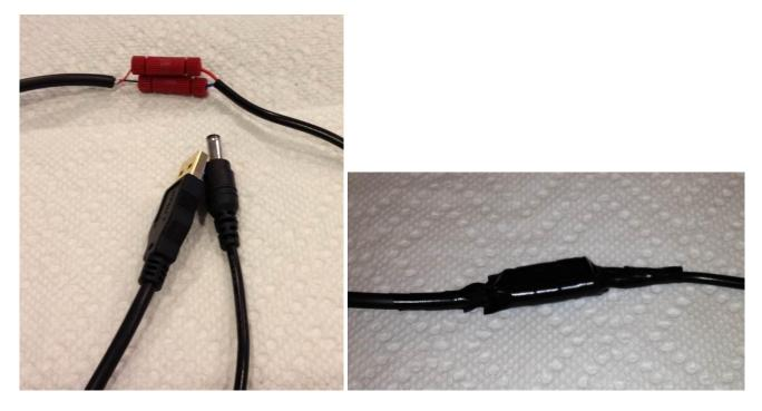
Finally, connect the new power cable to the HDMI converter and wrap some foam weather stripping around the metal to prevent rattles when it is tucked under the carpet. Be careful to avoid covering any of the vents.
