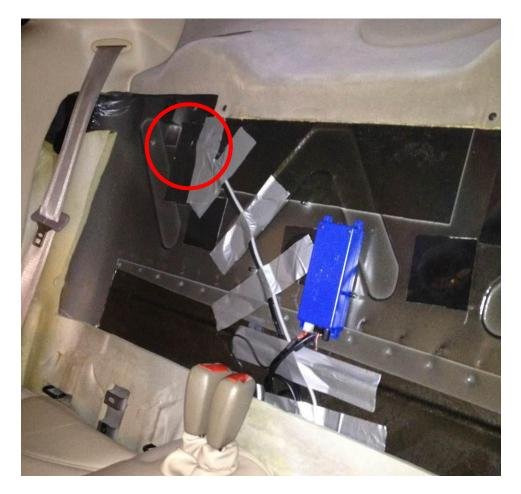
Next came the installation of the PIE APL/AI-AUX audio input which connects to the Alpine audio network between the navigation system and the amplifier and it was at this point that I went through several rounds of installation and modification to get the audio portion to work correctly. I will give some explanation of the problems and describe what the final solution ended up looking like.
