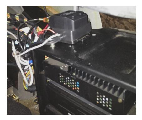
Once reassembled everything is in a tidy package that can be mounted on top of the frame that supports the audio amp using double sided automotive molding tape.
