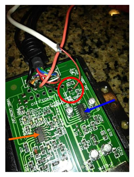
There is a conveniently located trough hole connecting the Q2 transistor to a trace on the back side of the board. I used this as the solder point for the switching wire (red circle). I also severed the trace connecting the timing circuit to the input side of the transistor (orange arrow). This probably isn't necessary but it ensures that the audio signal is completely isolated from our 12V switching signal.
