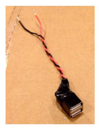
We now need a power cable for our HDMI converter box. I wanted to retain the plug in option so dug up an old USB cable and lopped the end off. Pulling out the red and black wires (pins 1 and 4) we now have one half of a plug in power cable for the 5V power outlet we made earlier.
