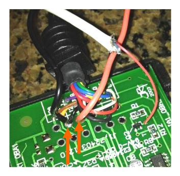
The audio switching is the reason for using Input #2 on the VCI-X, because when input #2 is active there is +12V applied to the center pole of the video selector switch. If you tie into the center pole of the switch and connect that to the audio toggle signal, then whenever video #2 is turned on, then the audio switches as well.
