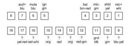
The space is a little tight and there are two things to connect but we want to tie in to the green ignition wire and the black ground wire. I opted to use the smallest splice (red) with a short length of wire and the next size up union (blue) to more easily accommodate the two wires needed to power the VCI-X and the HDMI converter.
