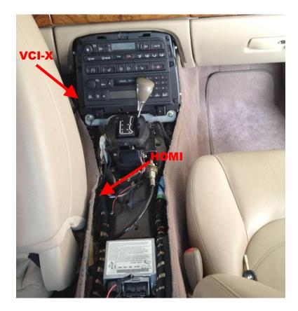
By removing the plastic retainer the console carpet can be pulled back and the VCI-X can be tucked up behind the radio support structure.
