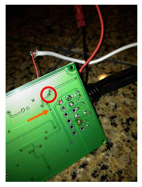
The PAC LD-10 pre-amp requires a +12V and GND be connected. It doesn't draw much current and since the AI-AUX box was already apart, I thought I would tie in to the power connections. Both the +12V and GND are available in the AI-Net cable so once the LD-10 is tied in to the AI-AUX, it will be a self-contained, plug in unit and won't need any splicing at all.
