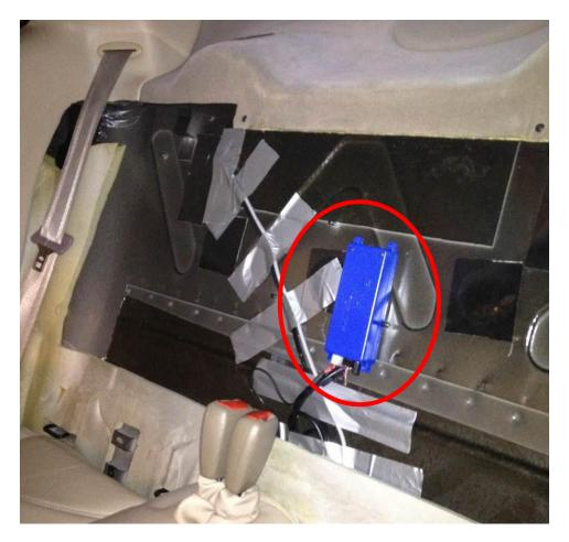
With the seat out, you can see 3 threaded studs in a triangle formation that would be used to mount the Jaguar phone module. These are pained and aren't easily visible in the picture. Looking at the back of the upper seat cushion there is a cut out in the center that the phone module would fit into. We can mount the Parrot box in this same location so that it fits into the existing seat cut out. The Parrot module is somewhat smaller than the Jaguar one so location isn't too critical.
