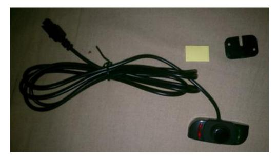
In the 2003 MY the connector in the console is an 18pin AMP 070 style (P/N 173853).
