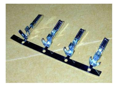
Strip the wires from the audio harness, the power harness and the half of the mic cable with the headphone like connector. Once this is done we need to affix one of the female pins to the end of each one.
