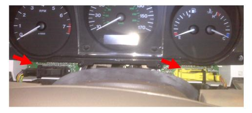
) Pull the dash unit out enough to flip and expose the reverse side and access the bulbs
