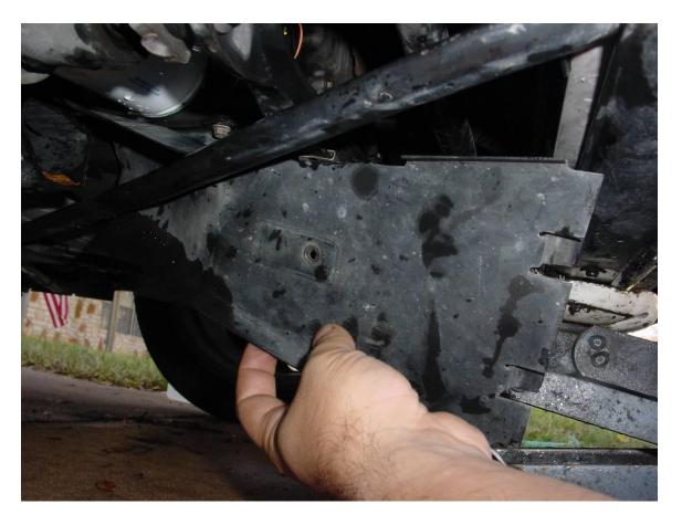
... and with the duct removed, we can now see the radiator drain plug (at right in the picture). This is on the right-hand end of the radiator on the engine side.
