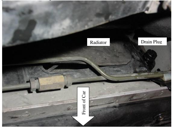
**Step 5**) \*ENGINE MUST BE COOL\* (switch ignition on and make sure temperature gauge is showing \*at most\* in the "blue" region, then turn ignition off).
