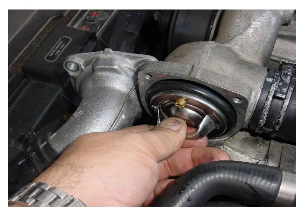
Step 25) Install cover and torque bolts to 8-10 Nm (6-7.4 ft-lbs).
