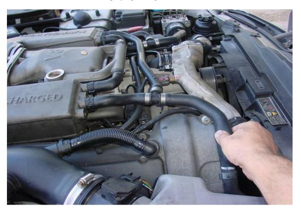
\*\*\*Step 17) Using the tool made in Step 1, install intercooler coolant plug.
