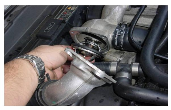
**Step 24**) Install the new thermostat with the air bleed valve (brass with ball bearing) at the top, as shown.
