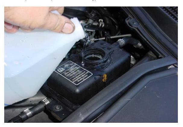
\*\*\*Step 10) ...and add clean tap water to intercooler plug until drain runs clear.
