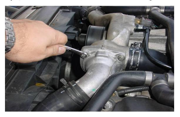
**Step 23**) Pull off housing cover. Remove and discard the old thermostat (or keep it for an "emergency" spare).
