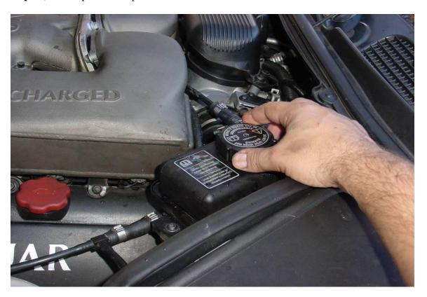
\*\*\*Step 16) Fill the system at the intercooler plug. You can "burp" air out of the system when the water level nears the top by squeezing the intercooler hose as shown.
