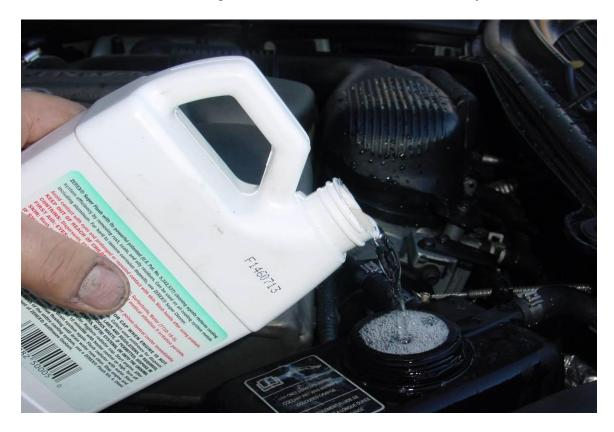
**Step 14**) With clean tap water, fill the system at the coolant tank. You can "burp" air out of the system when the water level nears the top by squeezing the radiator hose as shown.
