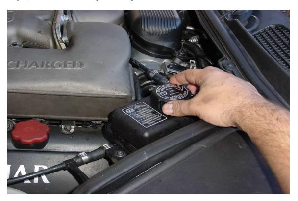
\*\*\*Step 8) Using the tool made in Step 1, remove the intercooler coolant plug.
