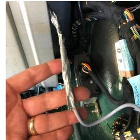
With top up, pull carpet from rear deck. Route cable under carpet and down passenger side back seat upright. I taped the cable to the body under the deck carpet.
