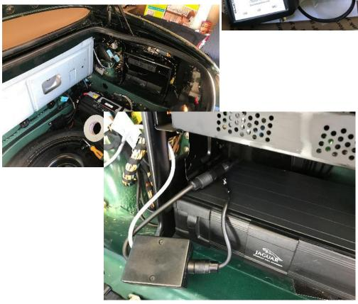
Wrapped long patch wire that runs to center console with duct tape for triple insulation in places where it will contact sharp edges.
