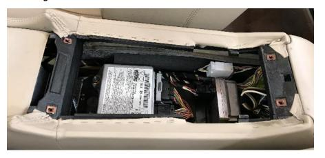
The cable is easier to route into the center console if you tuck the connector under the edge and pull it into place.
