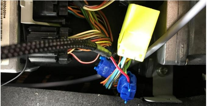
Bluetooth module tucked in and VHB taped to seatbelt tensioner metal box. Note that clearance is really tight under here. Watch your wire routing and make sure that your ashtray cover will open and close. Tie wrap or tape down all of your wires so they don't rattle.
