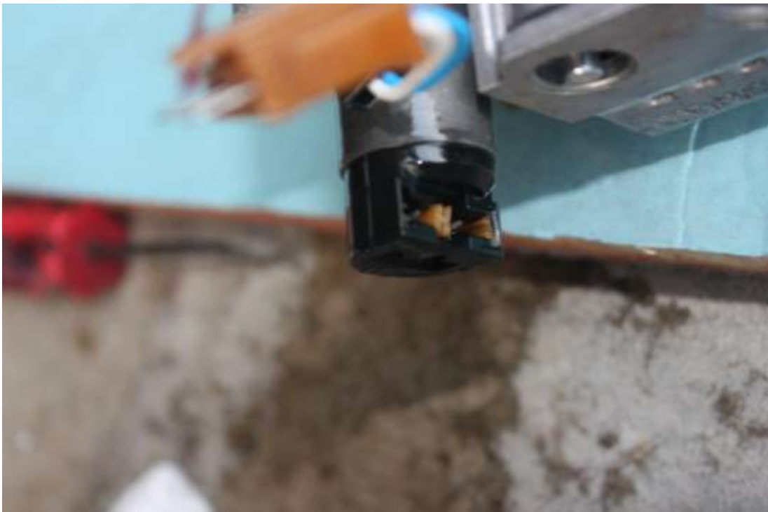
Figure 2 Bad Solenoid also broke off plastic in there from harness. I think i did it while inspecting it.
