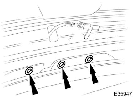
3. Remove the three blanking plugs from forward underside of trunk lid.
