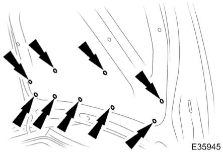
1. With trunk lid fully open, remove and discard fasteners securing liner to forward edge of lid.
