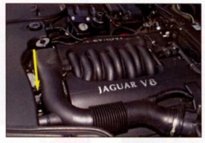
If a replacement engine has been fitted, a green tag should be visible down towards the back of the right-hand cylinder head.
