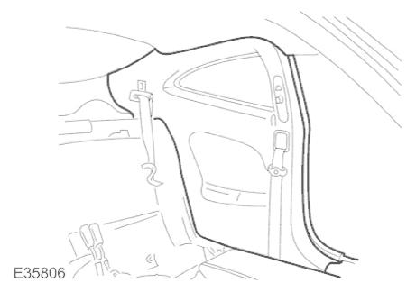
4. Position rear seat belts for access and remove squab from vehicle.
