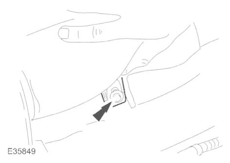
2. Slacken and remove the two rear seat squab securing screws.
