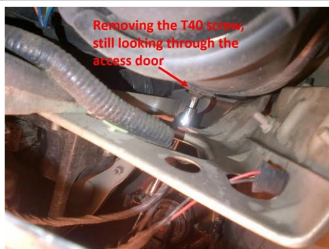
Using the combination of 1/4" socket wrench, 1/4" socket & extension and the T40 hex bit, put your arm through the access hole and remove the screw. It's a cumbersome task, but not too bad. It's a bit irritating because you can only use one eye at a time to see the screw for this step.
