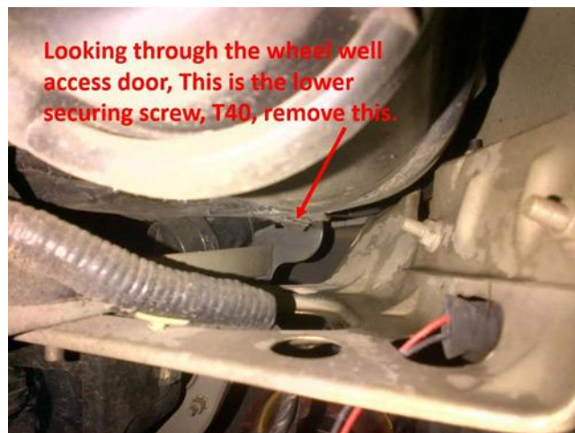
This is the T40 hex screw that holds the lens bottom of the assembly to the car. The removal of this screw is indeed the toughest part of this procedure.
