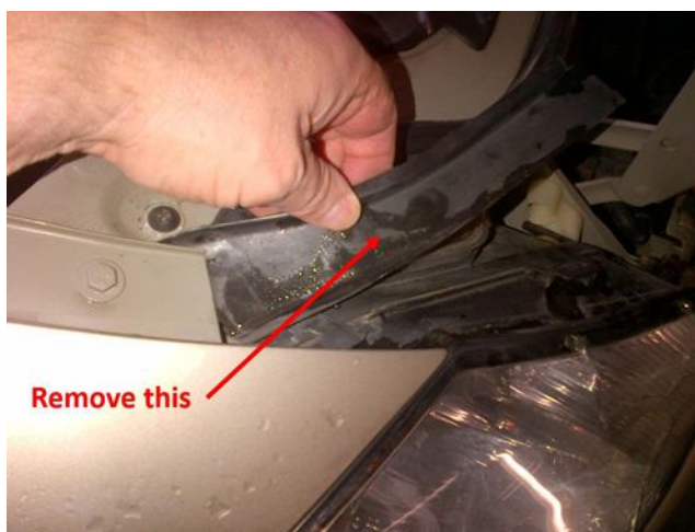
Remove the plastic cover, it just slides out. You may not have it, mine is missing from the other side of the car
