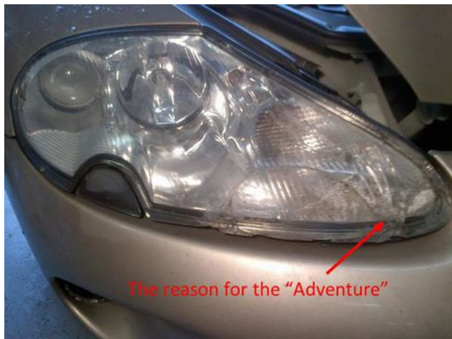
The reason for the adventure damaged XK8 XKR headlamp lens caused by stone damage
