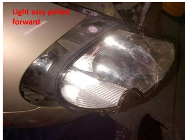
Carefully "wriggle" the headlight assy forward.
