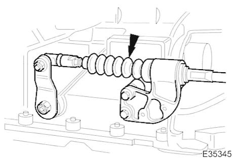
The gear selector at the transmission unit:
