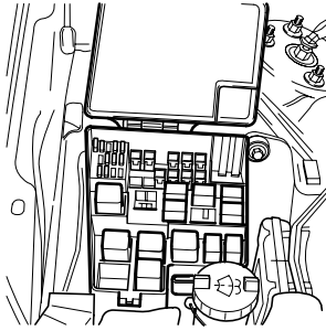
FRONT POWER DISTRIBUTION FUSE BOX
