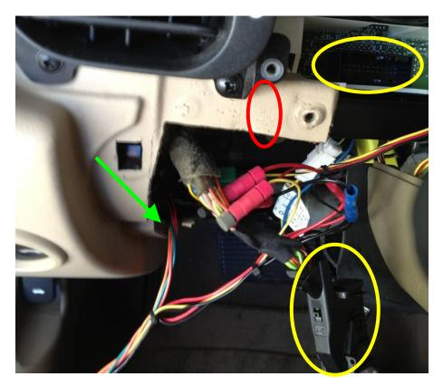
Of the five wires coming up from the lower part of the dash, three continue on to the A-pillar: switch, light, and pressure signal. The other two, power and ground for the pressure sensor, need to be connected here under the dash.
