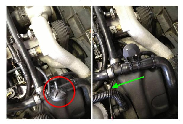
I routed the boost gauge harness along the breather tube to the back of the intercooler and then tied it to the small wire harness the runs across the top of the engine.
