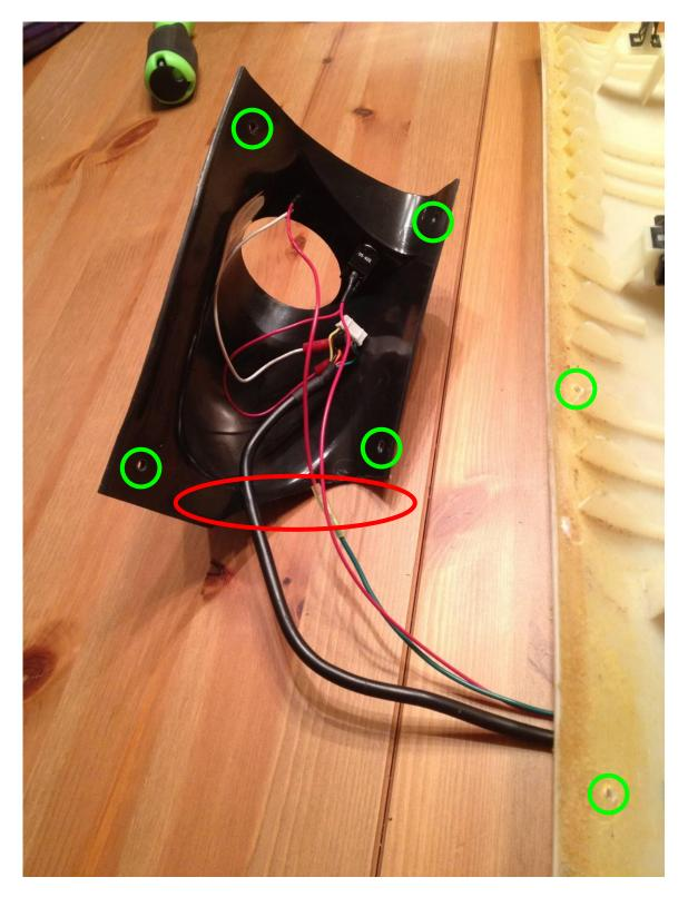
Now I attached the gauge pod with the screws, connected the gauge to the harness and fit it together for the first time. I didn't glue the gauge pod down just yet, because I wanted to install it in the car and make sure everything worked properly.
