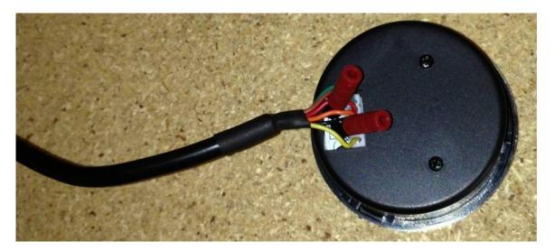
The switch I chose is a push on / push off type, that mounts through a  $\frac{1}{4}$ " hole. Just about any kind of switch will work since the current is so low, but this one took up the least amount of space and was not too intrusive to the interior.
