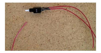
For the LED, the white wire (ground) can be directly connected to the Posi-Tap and the red wire will need an extension to make it long enough to route out of the pod and easily connect behind the A-pillar trim.
