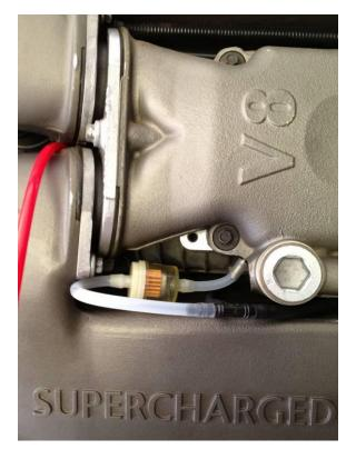
The pressure sensor is fairly small and for lack of a better place, I just strapped it to one of the intercooler coolant hoses. I connected the tubing and turned it downward so that it wouldn't interfere with the hood liner.
