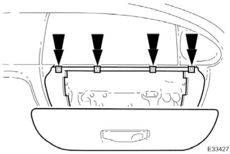
1. Open glove box lid and slacken and remove four screws securing liner to the fascia.
