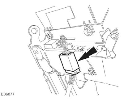
6. Position front seat for access, disconnect seat harness multiplug and remove seat from vehicle.
