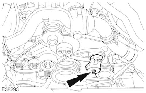
1. To install, reverse the removal procedure. 1. Tighten to 40 Nm.
