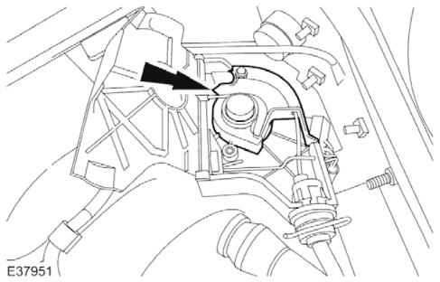
9. Make sure the APP sensor cam is at the idle position.
