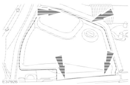
2. Remove the driver side bulkhead cover.
