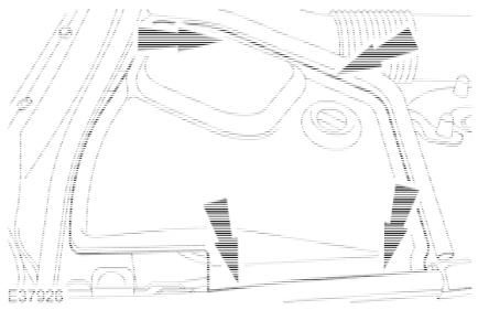
12. Install the driver side bulkhead cover.
